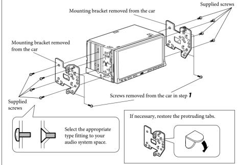
Note : When installing the unit on the mounting bracket, make sure to use the supplied screws (M5 x 8 mm). If longer screws are used, they could damage the unit.
